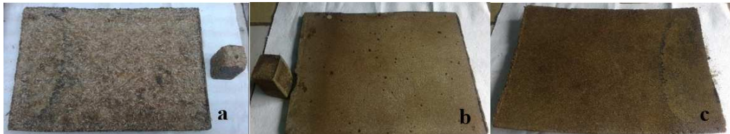
Photography 1: CNMLK Board. No Milled Rice Husk Board with Kraft Lignin (a). CMLP Board. Milled Rice husk Board with Resin of Depolymerized and Hydroxymethylated Lignin (b). CMLK Board. Milled Husk Board with Kraft Lignin(c)
